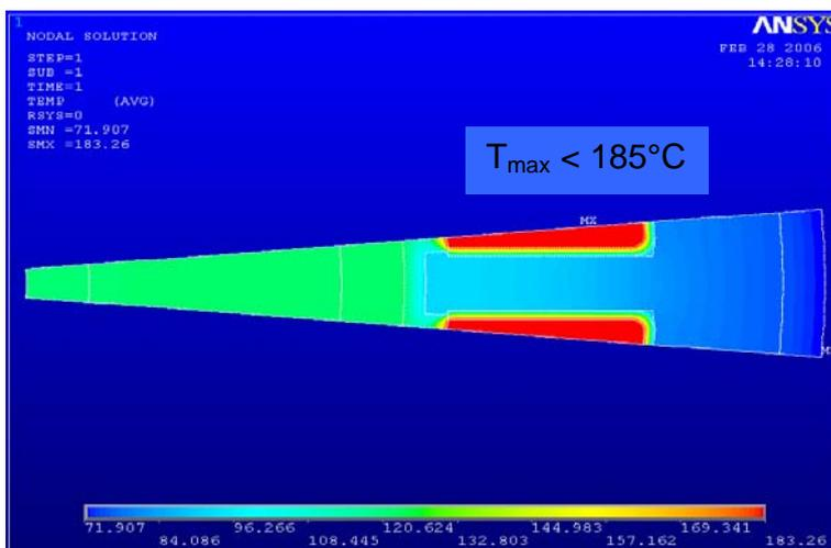
Figure 9: Temperature calculation of a high-speed electric motor calculated using ANSYS (long-term torque capability: 34Nm).
