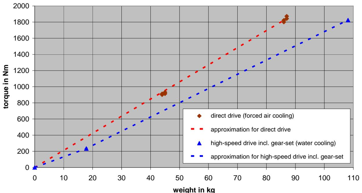
Figure 12: Torque versus weight characteristics of the different wheel-hub drive alternatives.
