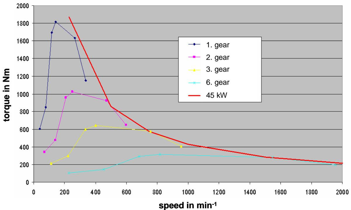
Figure 7: Torque-speed-characteristic at the wheels of a typical mid-size passenger car.
