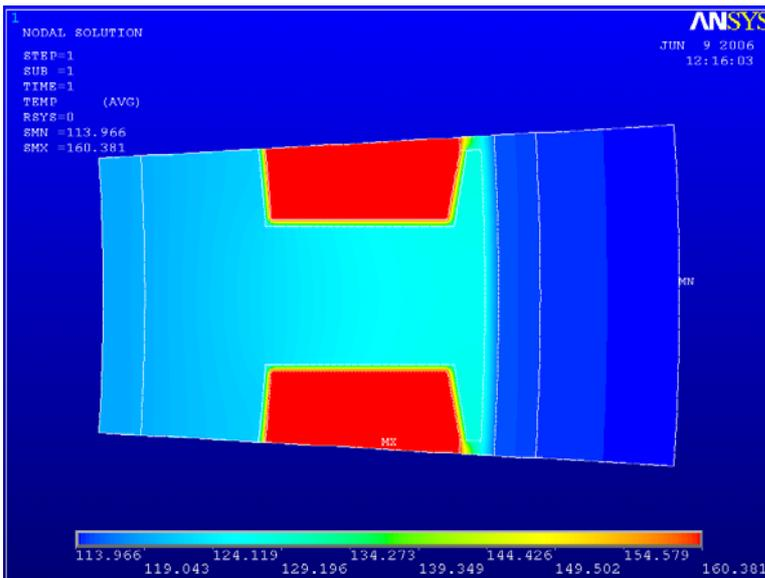
Figure 11: Temperature calculation of a low-speed direct drive electric motor calculated using ANSYS (long-term torque capability: 350Nm).
