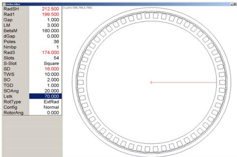
Figure 10: Geometry of a low-speed direct drive electric motor calculated using SPEED.
