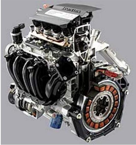
Figure 2: Honda Civic IMA system, electric motor shown in the front [2].
