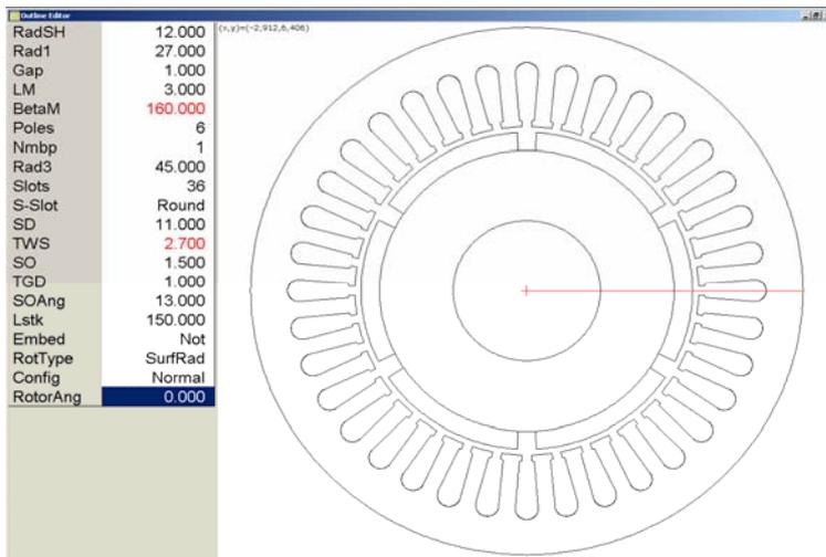
Figure 8: Geometry of a high-speed electric motor calculated using SPEED.
